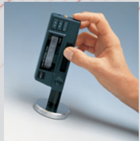
Hardness testing on a hardened work-piece
